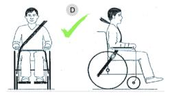
Tighten the restraint belts as much as possible, while ensuring the user's comfort.
