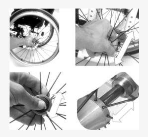
Grasp the wheel by the spokes around the hub, press the release pin button with your thumb and, without releasing, extract the wheel fully.
