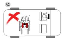
5. The wheelchair should be secured by a tie-down restraint system according to ISO 10542 or SAE J2249 with non-adjustable front straps and adjustable rear straps using Karabiner clips or "S" hooks and buckle fittings.
