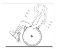
To find the point at which the chair will tip back easily and, consequently, to find the safe manoeuvring range, proceed as described below.
